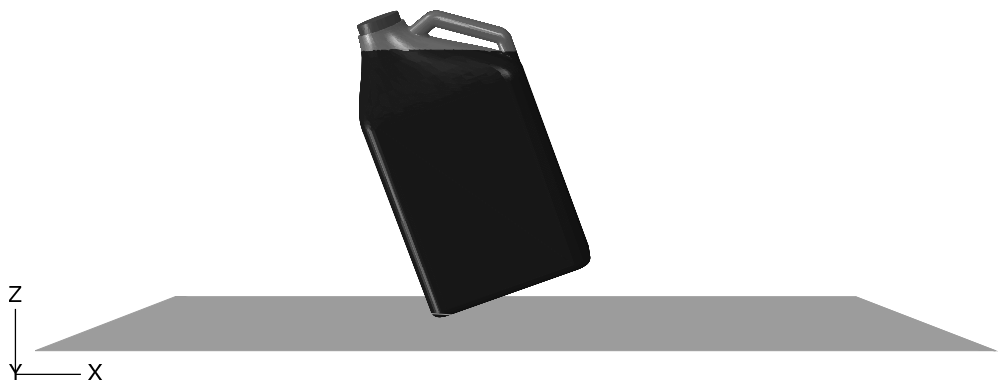
Figure 2.3.2–2 Assembly of the bottle drop model; the water is instanced inside of the bottle.
