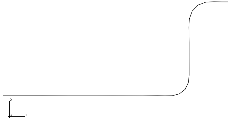
Figure 1.3.7-3 Deformed configuration after the first forming stage.
